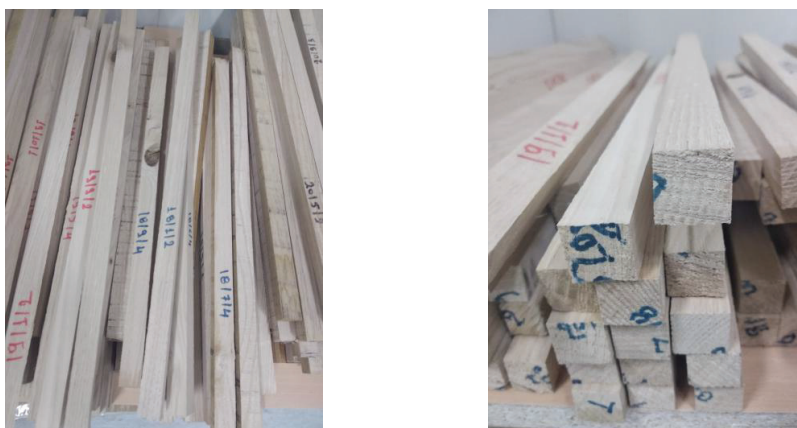
Figure 1. Chestnut wood specimens with collection-date code marking (a) and detail of their cross-section (b), prior to cutting to final test dimensions.
