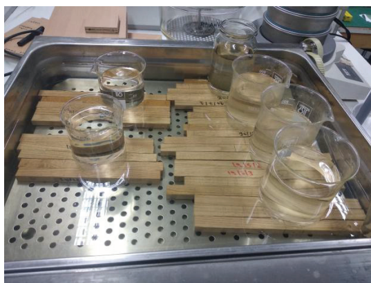
Figure 3. Chestnut wood specimens during immersion in water, as part of the water absorption and swelling test.
