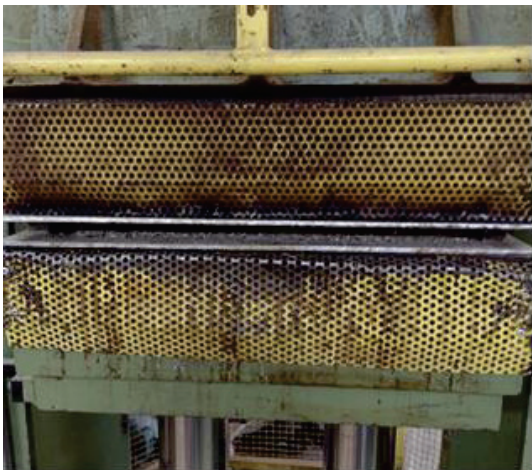
Figure 3. Production of a sunflower husk particleboard in a laboratory press
