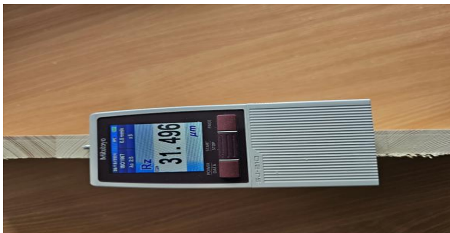
Figure 3: General view of the profilometer model SurfTest SJ-210 during measurement (Mitutoyo, Japan)
