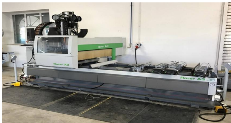
Figure 1: General view of the CNC woodworking milling-drilling center, model A3.30 (Biesse, Italy)
