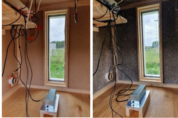
Figure 4: Inside the models in Uppsala, Sweden. Control model with medium density fiberboard (MDF) as wall material and ordinary floor (left), and the model reinforced with new wallboards and floor with PCM (right).
