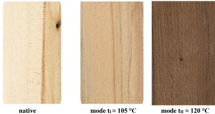
Figure 1: Wood color of unsteamed beech wood with false heartwood (native) and steamed beech sapwood with false heartwood by individual steaming modes after unification of color.
