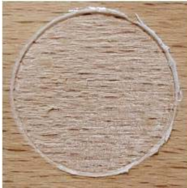
Figure 2: A test specimen after a pull-off test
