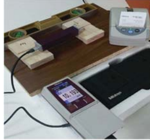
Figure 2: Roughness measurement with portable linear instrument
