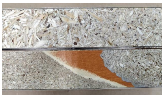
Figure 5: Defects when cutting an element with longitudinally oriented details in the core
