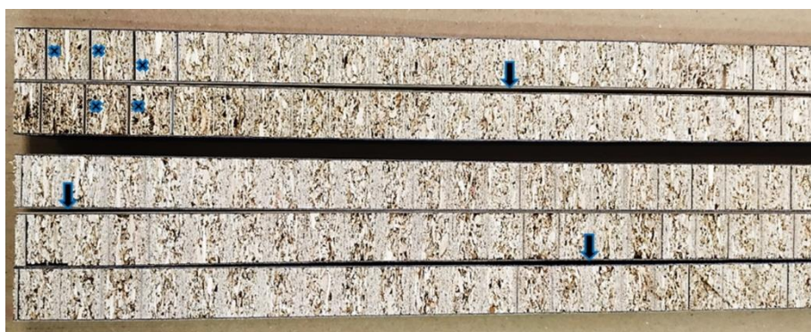
Figure 4: Defects of the specimens: ↓ – the element warping; * – holes, as a result of rotation of the core details
