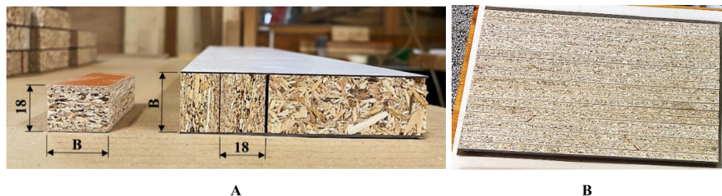
Figure 2: Schematics of core detail arrangement. A – orientation of the details, B – initial scheme of the detail arrangement
