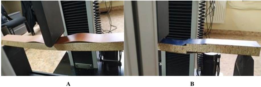
Figure 8: Damaging of specimens under bending stress. A – longitudinal orientation of the core details; B – transverse orientation of the core details
