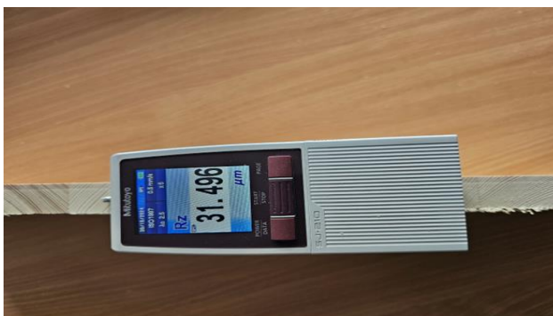
Figure 3: Portable roughness tester, model Surftest SJ-210 (Mitutoyo, Japan) during the measurement
