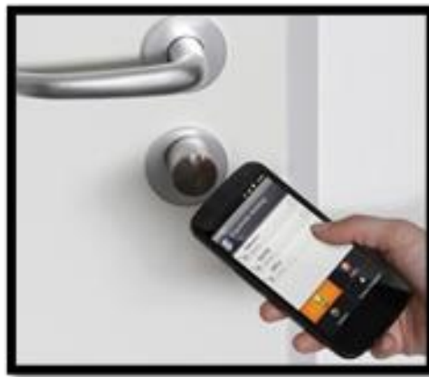
Figure 21: Smart phone access control
