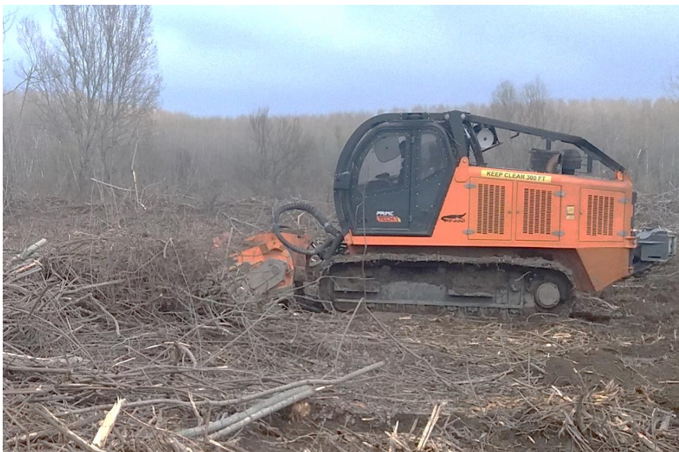
Figure 1: Self-propelled milling unit PT-400 with multi-purpose forestry milling machine FAE 300/S for complete soil preparation of poplar fellings (Photo K. Marinov).
