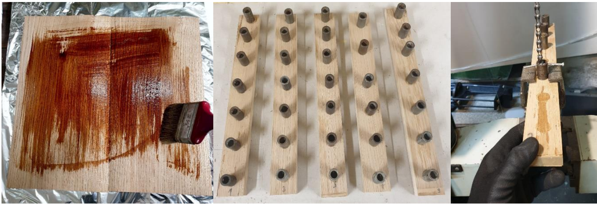
Figure 1: Applying the adhesive and testing the samples
