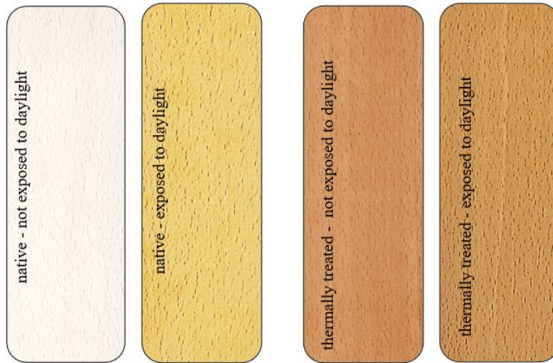
Figure 1: View of beech wood: (left) unsteamed before and after exposure, (right) thermally treated before and after exposure
