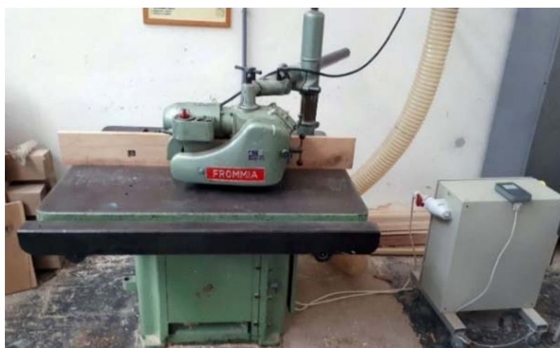
Figure 2: Lower milling machine FVS with feeder Frommia ZMD 252/137
