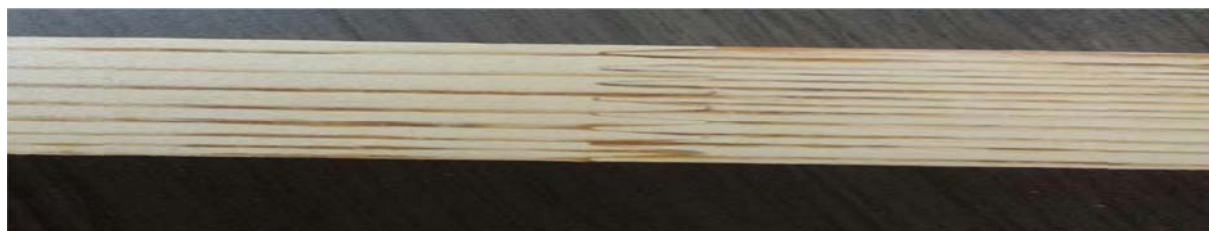
Figure 9: Finger joint pine with vertical teeth
