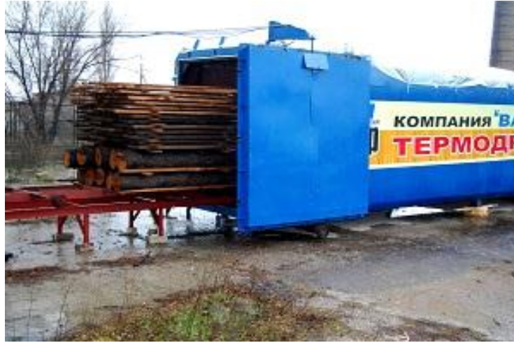
Fig. 1. The thermoconvective heat treatment dryer (Russian name – SPCT)
