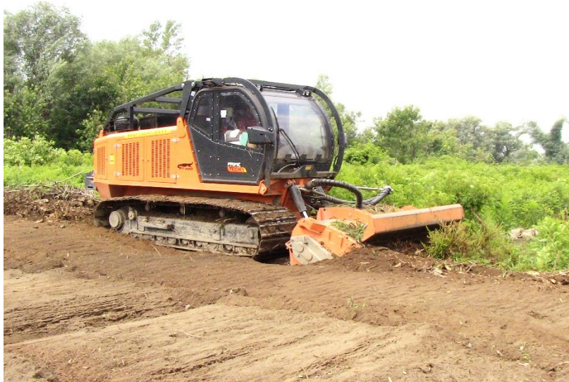
Figure 2: Stroke of specialized milling unit Prime Mover PT-400 with multifunctional forest cutter FAE-300 / S, in the first working section, State Forestry “Oryahovo”
