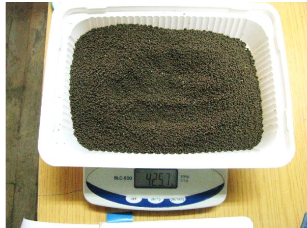
Figure 5: Determination of grain mechanical composition of soil samples
