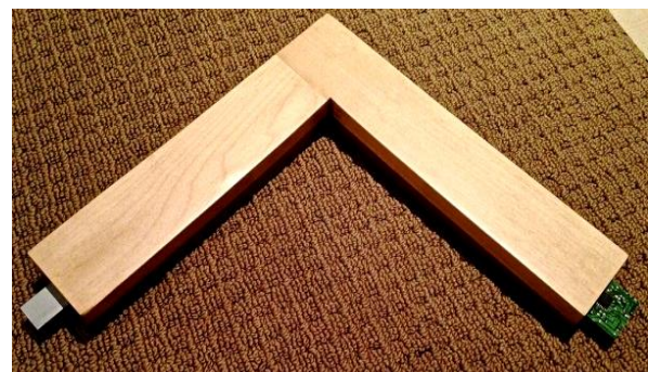
Figure 5: Electronics & metal cased in insulating wood.
