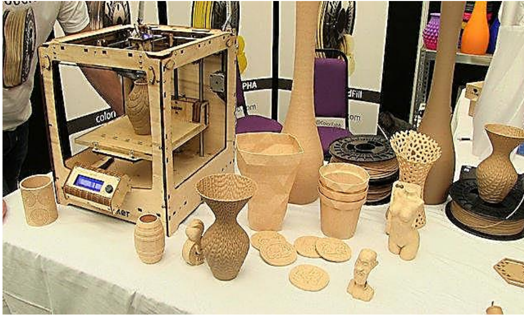
Figure 4: 3D wood printer and printed models from Laywoo-D3.
