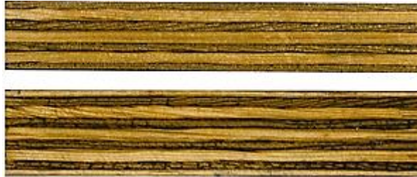
Figure 5: Test specimens of seven and nine-layer plywood models after 6 hours immersion in boiling water
