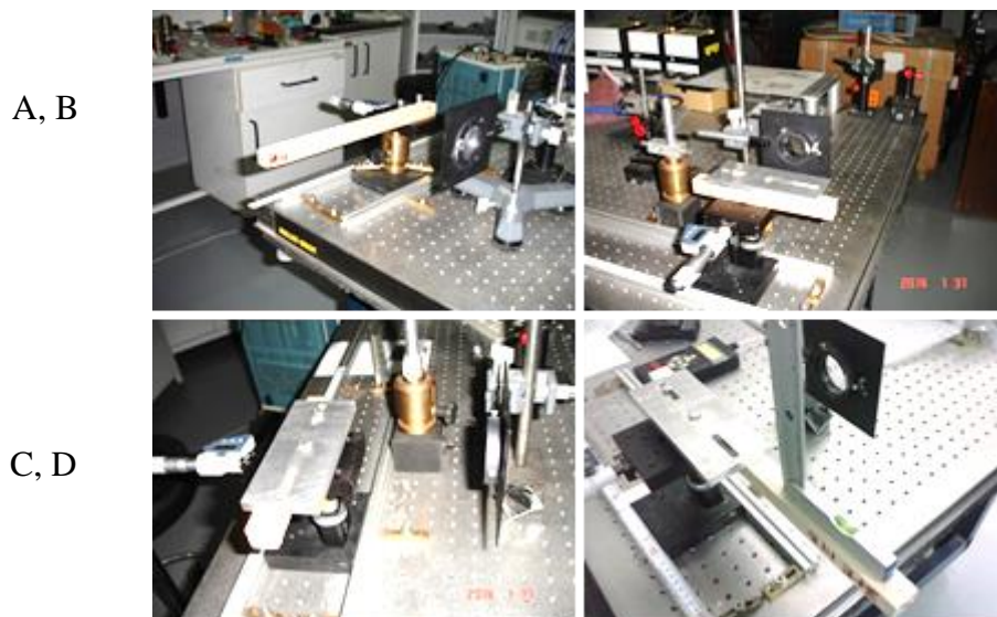
Figure 3: XYZ positioning system of wood specimens: a) front view (first row on the left), b) rear view (first row on the right), c) side view (second row in the left), d) top view (second row in the right)
