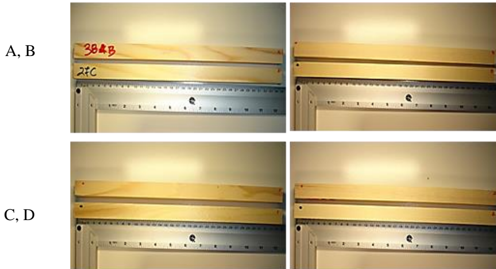
Figure 2: Wood specimens of fir (red) and spruce (blue) before drilling- tangential 1st side (first row on the left), radial 2nd side (first row on the right), tangential 3rd side (second row on the left), radial 4th side (second row on the right)
