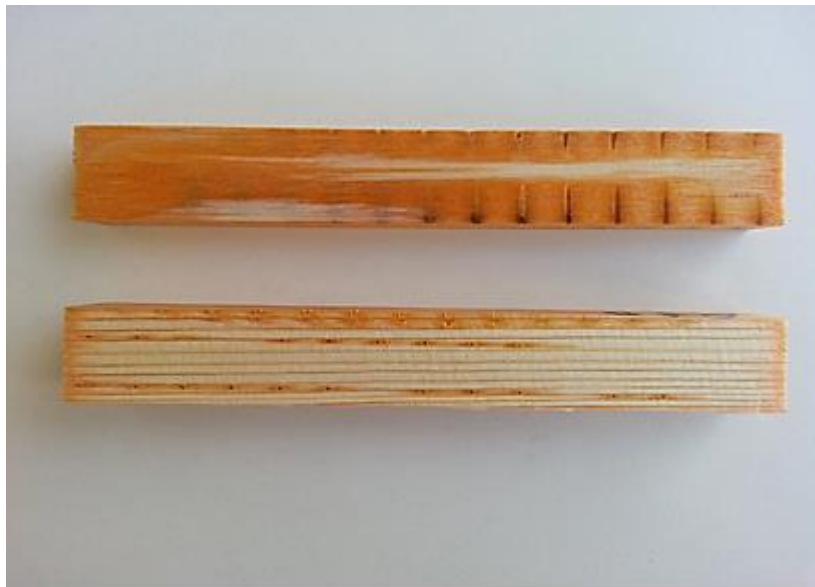
Figure 12: Penetration of rape oil axially and transversely in fir and spruce laser drilled wood specimens (see, also, the shape and depth of non-carbonized holes \sim 0.4 cm in depth).
