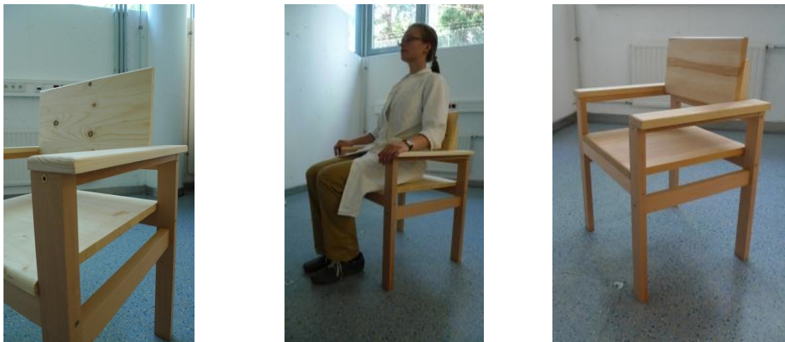
Fig. 1. Testing chair with exchangeable sets of seat boards, arm rests and backrests, arm rest are also usable for testing the edge radius preferences.
