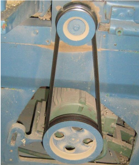
Figure 1: A planer driven by a V-belt
