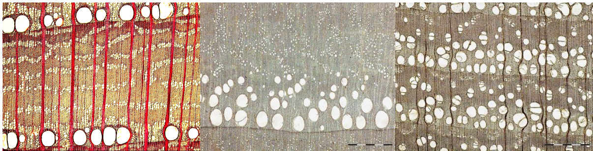
Figure 4: Distribution of early and late wood in the tracheas of Kalopanax , Castanea and Phellodendron
